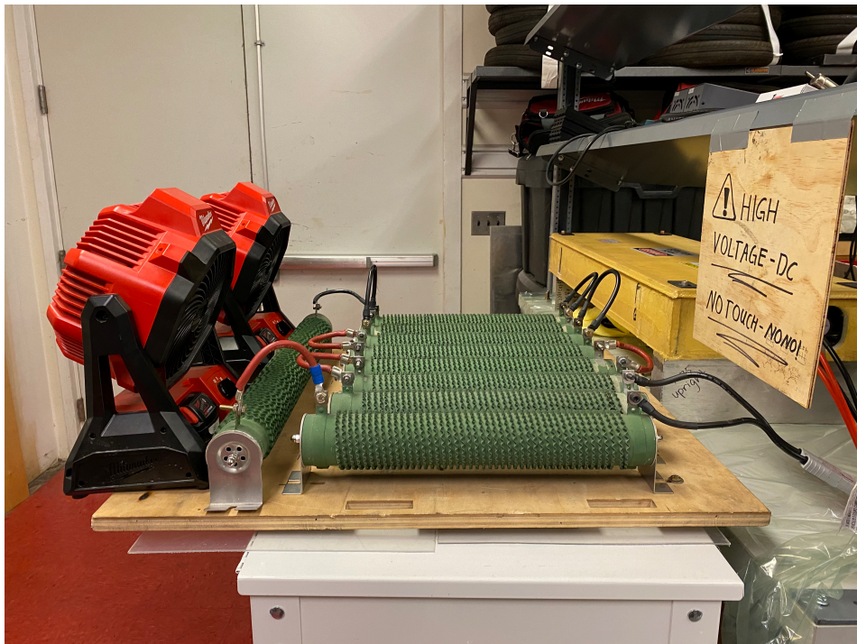
Image 1: Dashboard plugged into batter and resistor cooling exhaust fan on an electrically insulated table.
