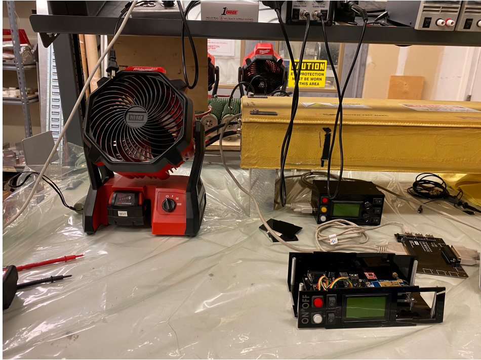
Image 1: Dashboard plugged into batter and resistor cooling exhaust fan on an electrically insulated table.
